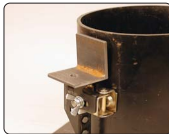
Angle Iron on large pipe
